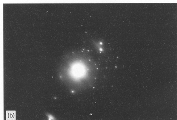
Figure 13 TEM of Al-Sibral fibres composite (a). Electron diffraction pattern (b).
